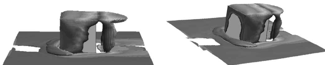
Fig. 6. Coherent structures visualised by vorticity magnitude at different perspective view angles.
